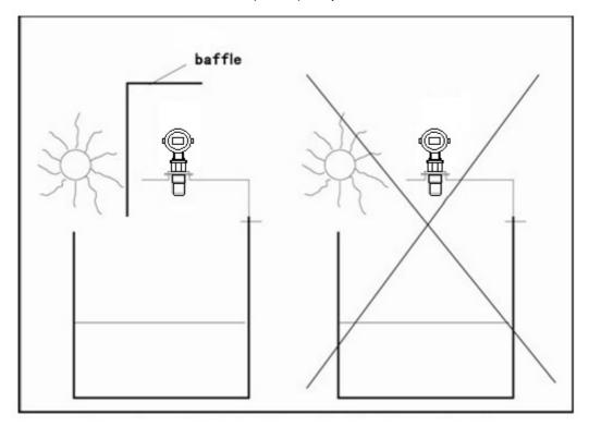
A sun shade or baffle, can be made from either sheet metal or plastic, customised for your application requirements. This can be fabricated by the customer or supplied by DAYTECH. Please contact DAYTECH if you would like custom sun shades manufactured.
