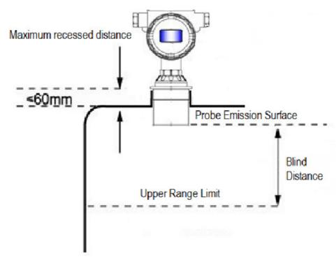
With flange installation, follow the below diagram. Ensure the probe's face is not recessed more than 30mm, maximum flange depth is 60mm. Ensure the diameter of the flange is greater than 100mm.
